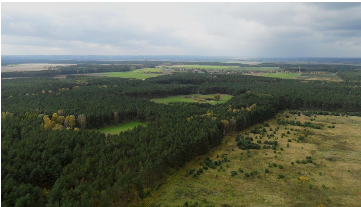
Figure 4: Example of a non-homogeneous roughness terrain in which a site-specific analysis concerning an appropriate measurement layout has to be performed to define the representativeness radius .
