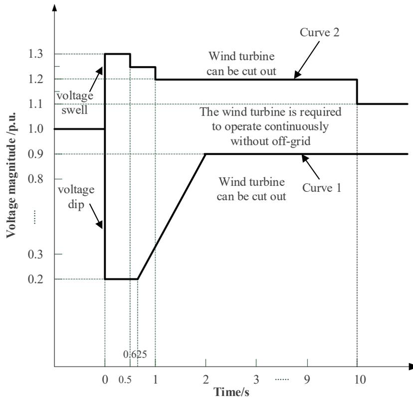
**Fig. D.1. FVRT curve of wind turbine**
