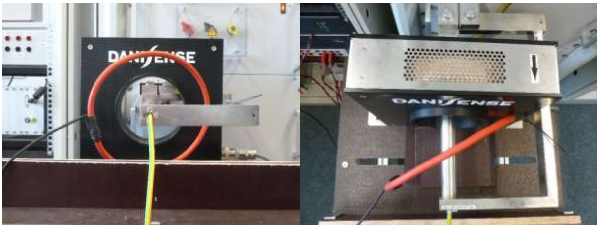
Figure 6: Example set-up: Calibration of a Rogowski current transducer in a centered position, but where the current transducer is not at right angle.
