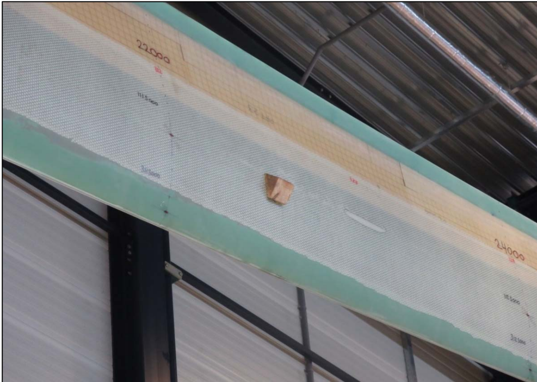
Figure 3 Impact point for excitation
