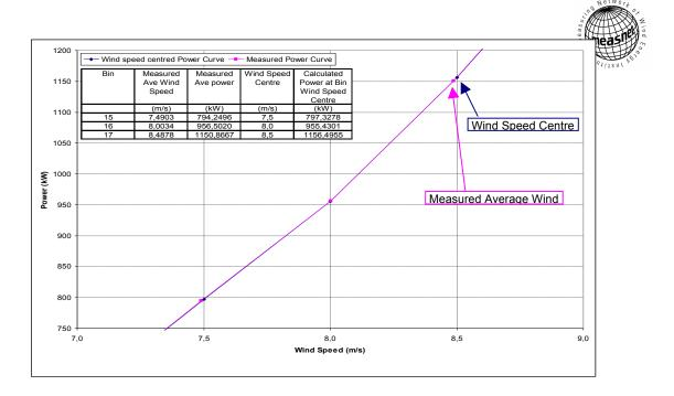
Once this wind speed centred bin power curve is obtained, the Site Specific AEP can be calculated by multiplying the value of the power at each bin by the hours at each bin in the site specific wind distribution.
